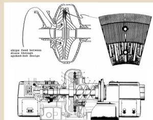
Figure 8. Technical drawing of possible pulper for use in the size reduction of husk fibers.
