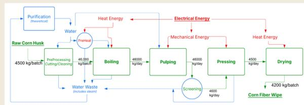
Figure 3. Process flow diagram for semicontinuous batch production of corn fiber-based wipes.
